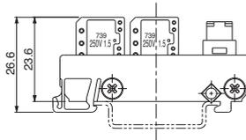
Notes: 1. The lengths in brackets are applicable when the junction terminal block is mounted on a 35 mm wide DIN rail.
