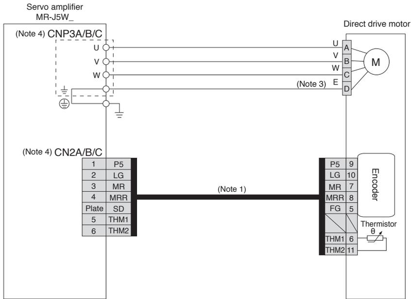
● For TM-RG2M/TM-RU2M/TM-RFM series (absolute position detection system)
