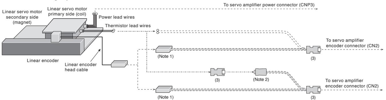
MR-J5-G-RJ/A-RJ and LM-F with a serial linear encoder
