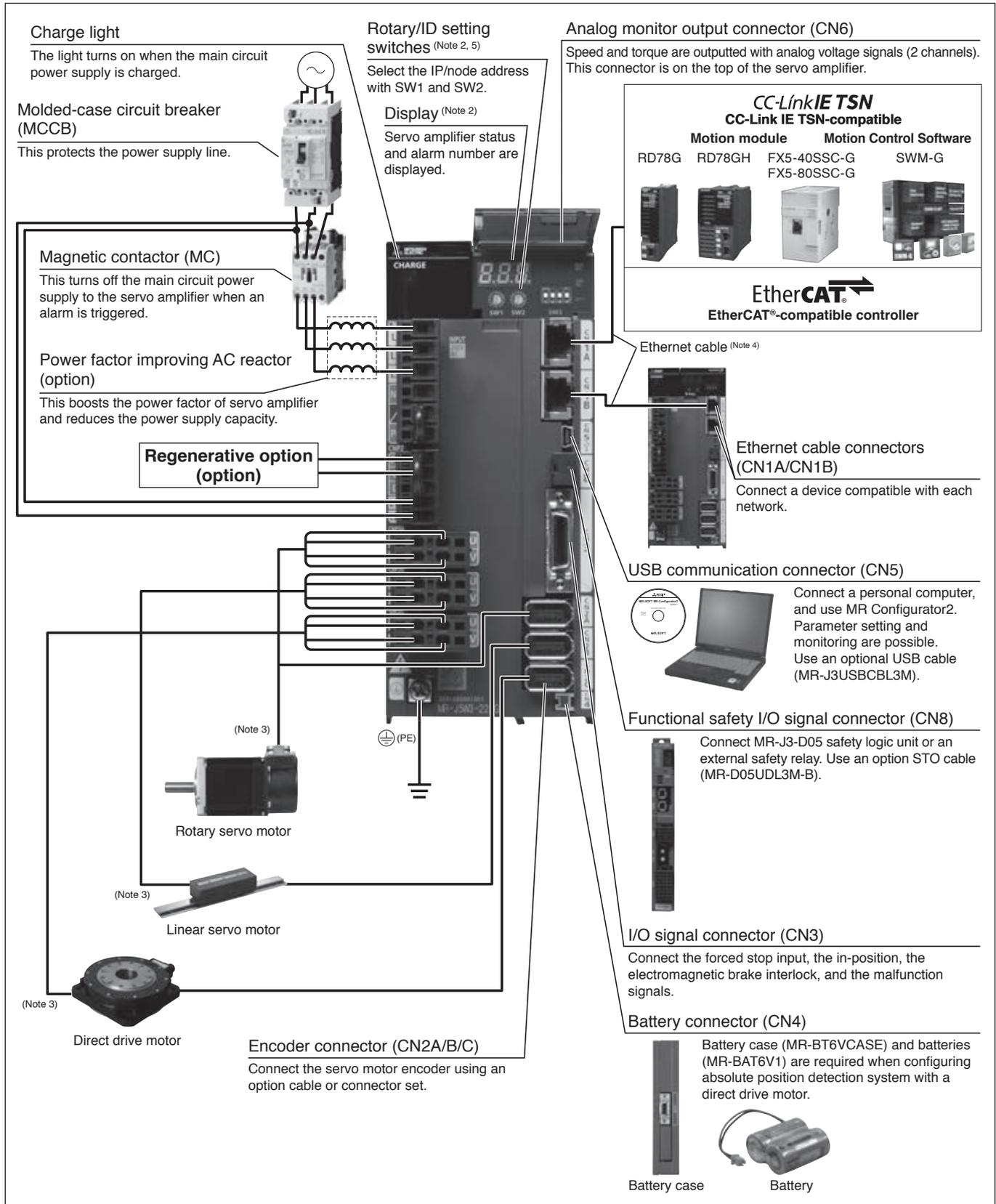
Notes: 1. The connection with the peripheral equipment is an example for MR-J5W3-222G(-N1). CNP3C and CN2C connectors are not available on MR-J5W2-G(-N1). Refer to "MR-J5 User's Manual" for the actual connections of each multi-axis servo amplifier.
