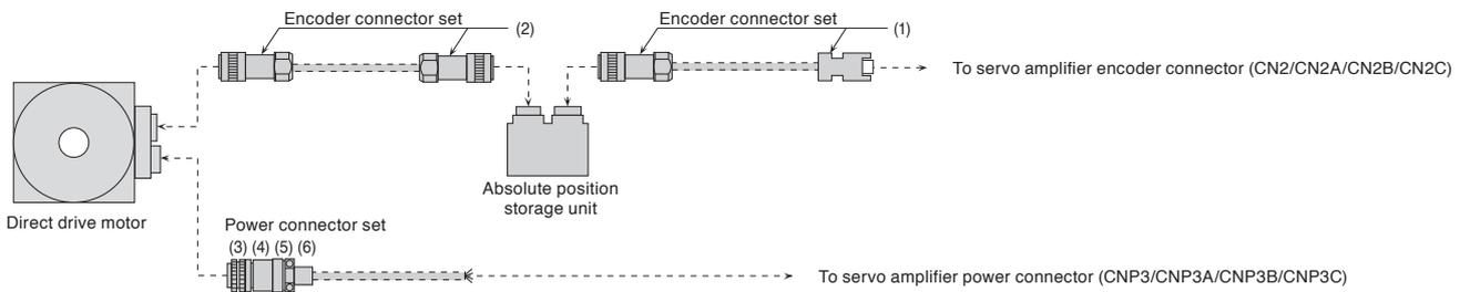
Notes: 1. Cables drawn with dashed lines need to be fabricated by users. Refer to "Direct Drive Motor User's Manual" when fabricating the cables.
