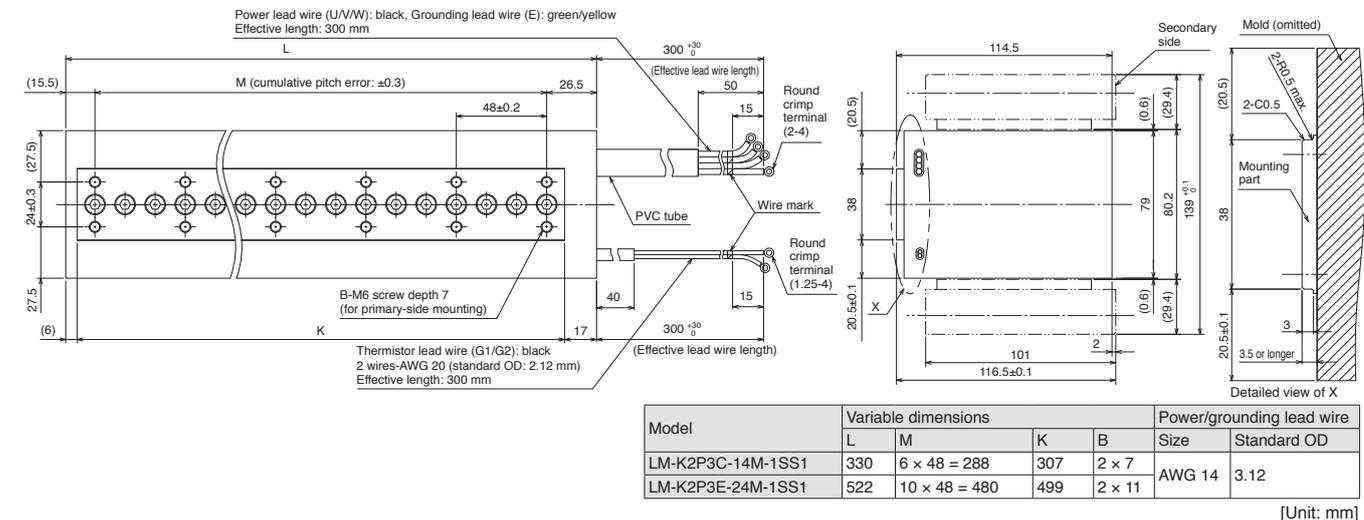
Notes: 1. Power, grounding and thermistor lead wires do not have a long bending life. Fix the lead wires led from the primary side (coil) to a moving part to prevent the lead wires from repetitive bending.
