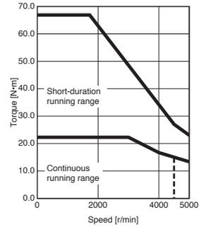
Notes: 1. Torque drops when the power supply voltage is below the specified value. - - - : A rough indication of the possible continuous running range for 3-phase 170 V AC
