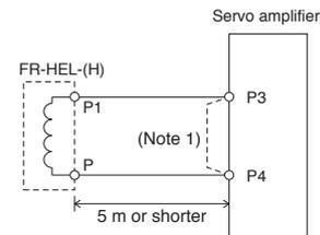
Notes: 1. Disconnect a short-circuit bar between P3 and P4 when using the power factor improving DC reactor.
