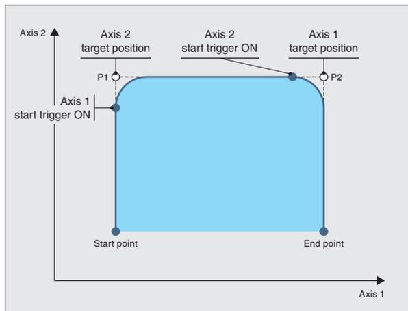
The triggered motion is a type of command that delays the execution of the motion command until the specified trigger condition is satisfied.
