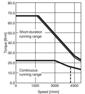
Notes: 1. Torque drops when the power supply voltage is below the specified value. - - - : A rough indication of the possible continuous running range for 3-phase 323 V AC
