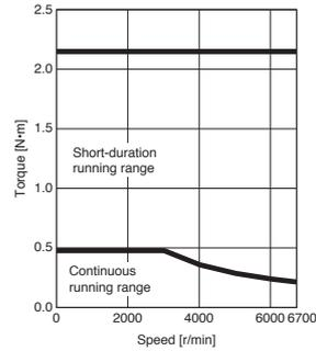
Notes: 1. Torque drops when the power supply voltage is below the specified value.
