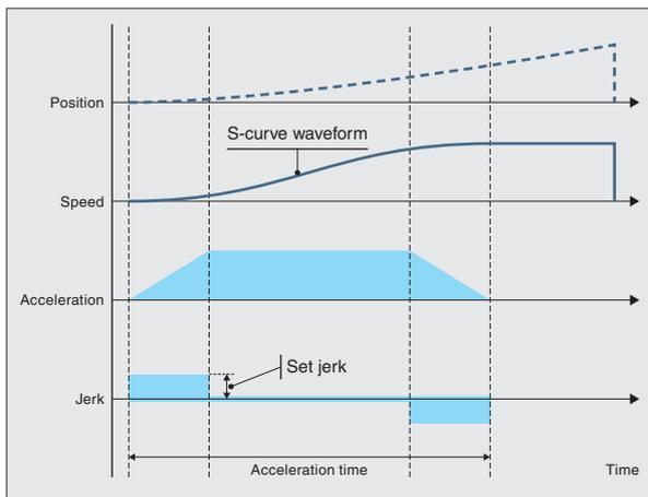
In this method, an axis can be accelerated gradually through adjusting jerk so that the vibrations of the machine can be minimized.
