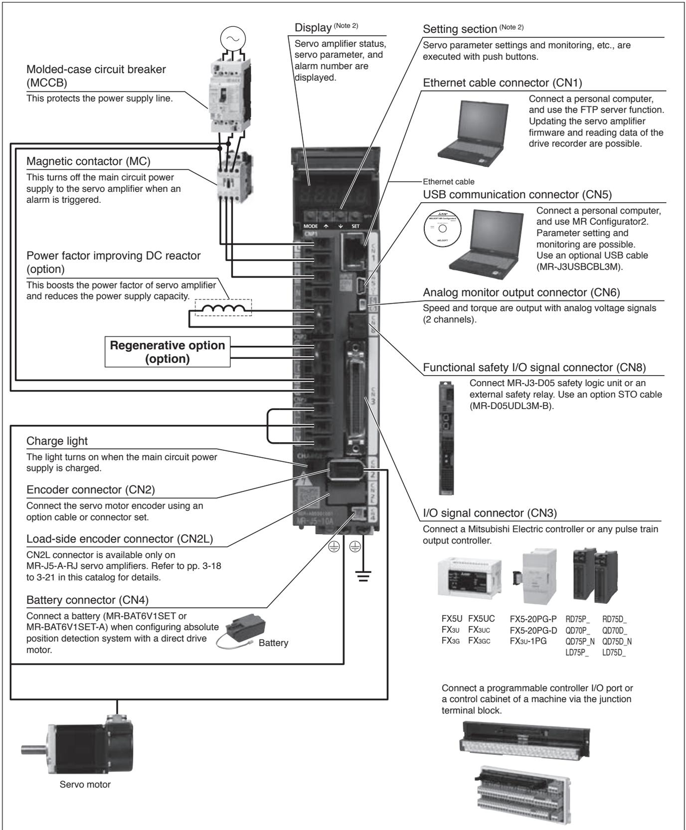
Notes: 1. The connection with the peripheral equipment is an example for MR-J5-350A(4)(-RJ) or smaller servo amplifiers. Refer to "MR-J5 User's Manual" for the actual connections.
