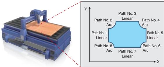
\*1. The multi-axis path control is possible using the buffer mode.
