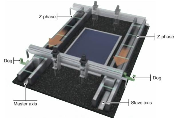
After the master and slave axes pass their respective dogs, the gantry home position return stops both of the axes at the Z-phase of the master axis. This method enables two or more axes to execute home position return simultaneously, supporting gantry systems.
