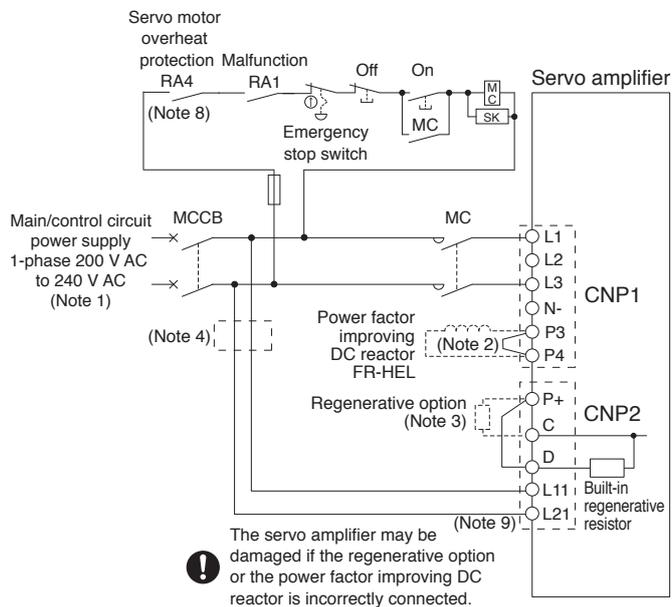
● For 1-phase 200 V AC and driving on/off of main circuit power supply with DC power supply
