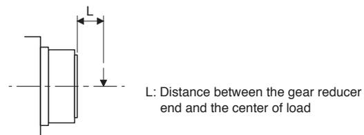
With a flange-output type gear reducer for high precision applications, flange mounting (G5)
