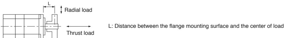
\*3. V10 indicates that the amplitude of the servo motor itself is 10 μm or less. The following shows mounting orientation and measuring position of the servo motor during the measurement:
