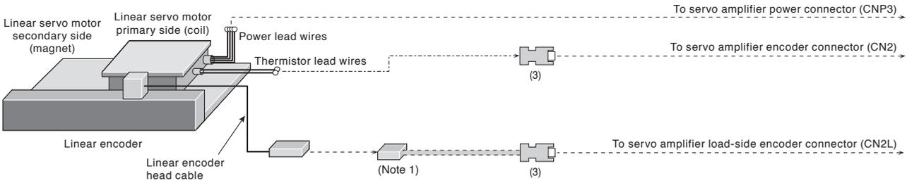
MR-J5-G-RJ/A-RJ and LM-F with an A/B/Z-phase differential output type linear encoder
