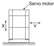
\*2. Refer to the diagram below for the permissible load for the shaft. Ensure that loads applied on the shaft do not exceed the values specified in the table. The values in the table are applicable when each load is applied singly.
