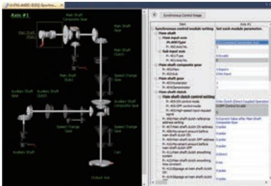
Synchronous control is executed by setting parameters of the input axis, output axis, gear, and clutch for synchronous control and turning on the synchronous control start signal.
