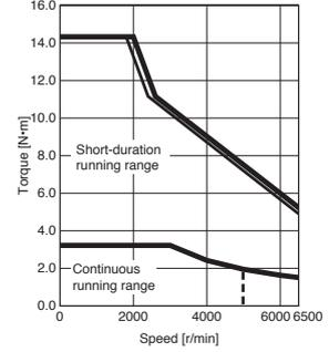
Notes: 1. Torque drops when the power supply voltage is below the specified value. - - - : A rough indication of the possible continuous running range for 3-phase 323 V AC
