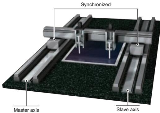
Motion Control Software enables tandem operation where the same commands can be outputted to master and slave axes.
