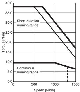
Notes: 1. Torque drops when the power supply voltage is below the specified value. - - - : A rough indication of the possible continuous running range for 3-phase 170 V AC
