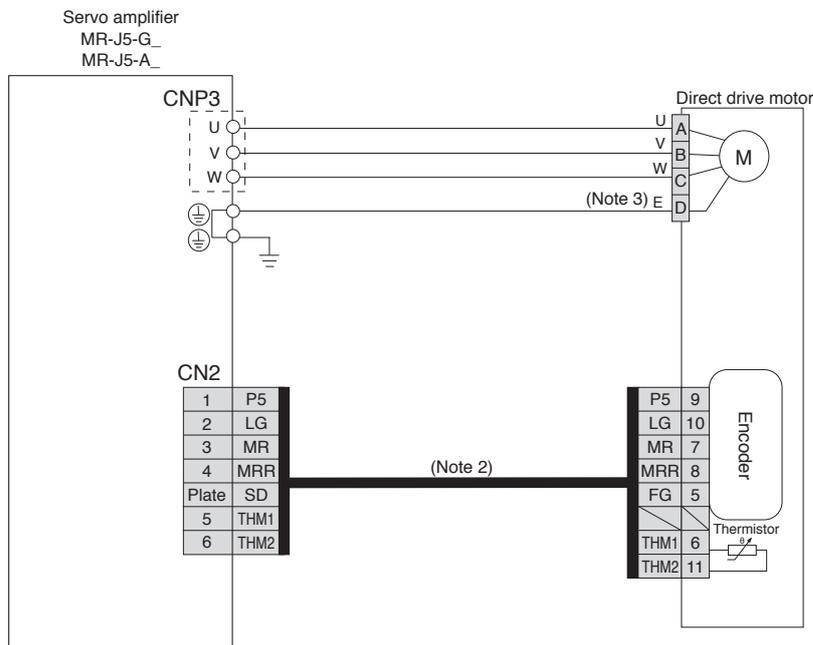
● For TM-RG2M/TM-RU2M/TM-RFM (absolute position detection system)
