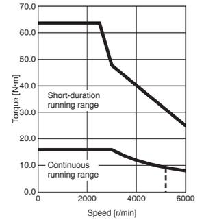
Notes: 1. Torque drops when the power supply voltage is below the specified value. - - - - : A rough indication of the possible continuous running range for 3-phase 170 V AC
