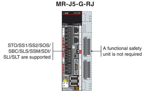
Servo motors with functional safety support the safety sub-functions at a higher safety level. The functional safety encoders provide the servo motor positions and speeds necessary for the safety sub-functions at a safety level of Category 4 PL e, SIL 3.
