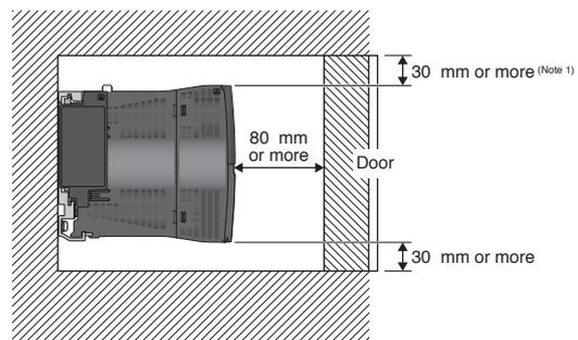
Notes: 1. Provide clearance of 30 mm or more when the height of a wiring duct is 50 mm or less. In other cases, provide clearance of 40 mm or more.
