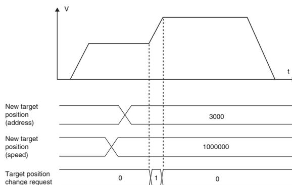
**Synchronous Control** Simple Motion
