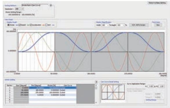
The cam graph can be flexibly and easily created through drag & drop. The waveform is changed according to the pointer's movement.
