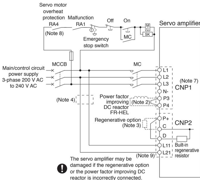
● For 3-phase 200 V AC and driving on/off of main circuit power supply with DC power supply
