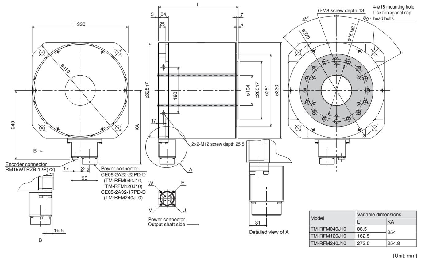
Notes: 1. General tolerances are applied to the dimensions in which tolerances are not given in the drawing. The actual dimensions may be 1 mm to 3 mm larger than the dimensions indicated. Make allowances for the tolerance when designing a machine.
