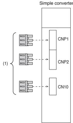
Connectors for daisy chain wiring (Note 2)
