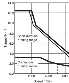
Notes: 1. Torque drops when the power supply voltage is below the specified value. - - - : A rough indication of the possible continuous running range for 3-phase 170 V AC
