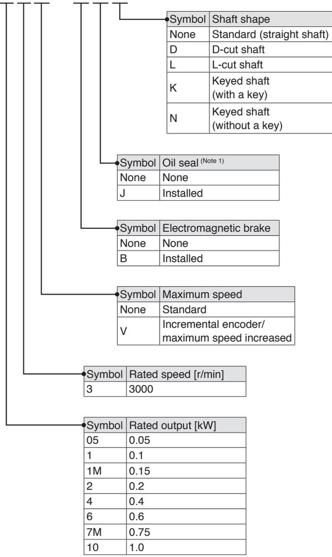
Notes: 1. The dimensions are the same regardless of whether or not an oil seal is installed.
