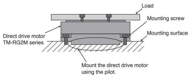
● Table type (with positioning pin holes)
