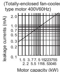
For "Δ" connection, the amount of leakage current is approx. 1/3 of the above value.
