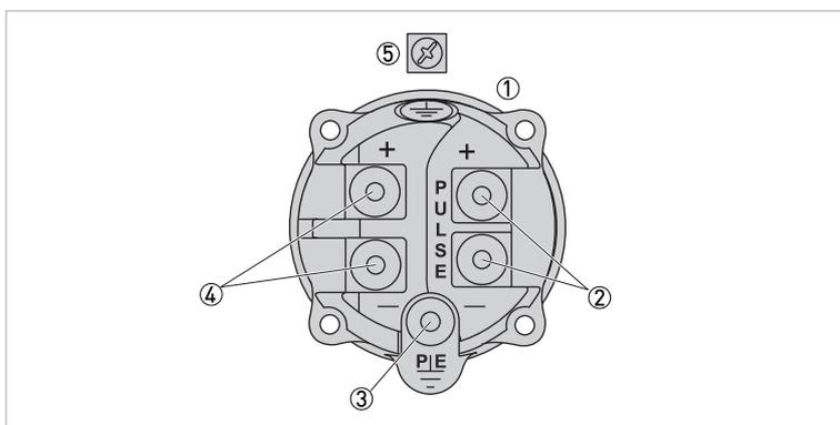
**Figure 4-1: Identification on field terminals**
