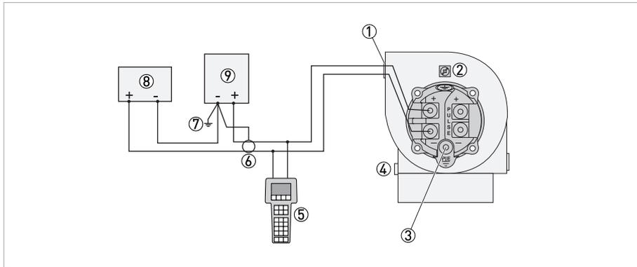
Figure 4-3: Wiring a flowmeter with a 4...20 mA output
