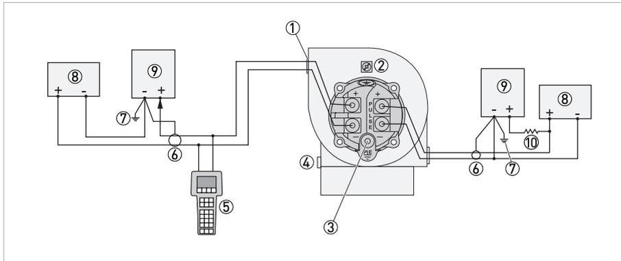
Figure 4-5: Wiring a flowmeter with a pulse output transistor switch (sinking) counter input with external power supply and pull-up resistor
