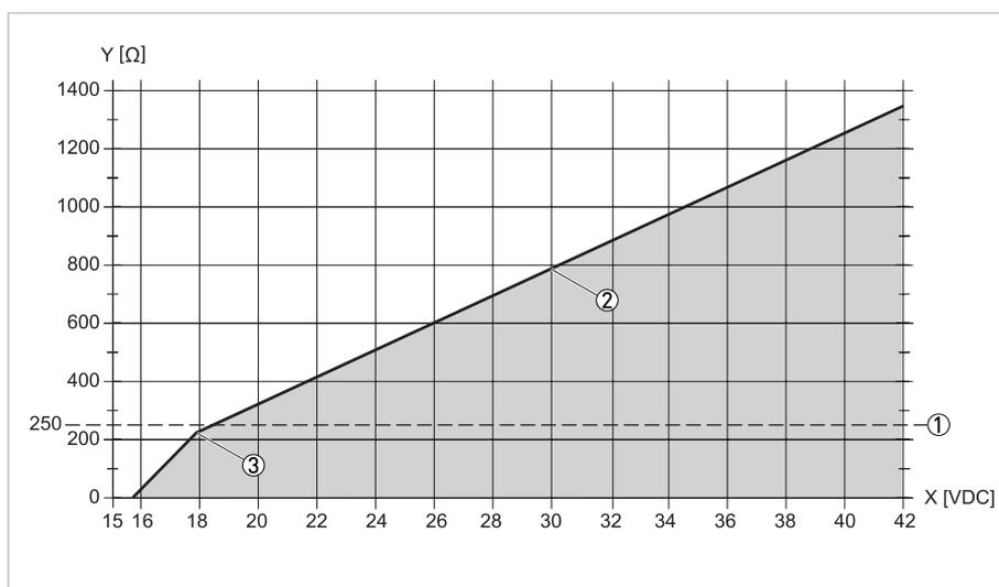
Figure 4-2: Relationship of output load versus supply voltage
