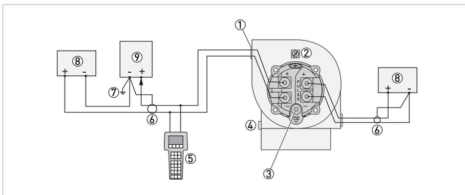
Figure 4-4: Wiring a flowmeter with a pulse output transistor switch (sinking) counter input with receiver supplied power
