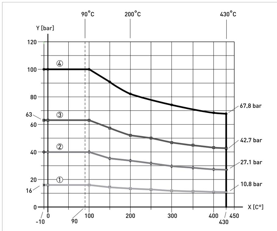
Figure 2-3: DIN flange rating acc. to EN 1092-1 for material group 14E0
