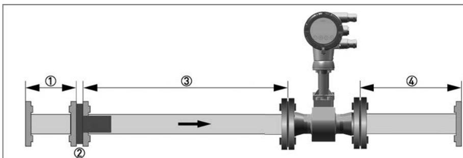
Figure 3-8: Flow straightener
