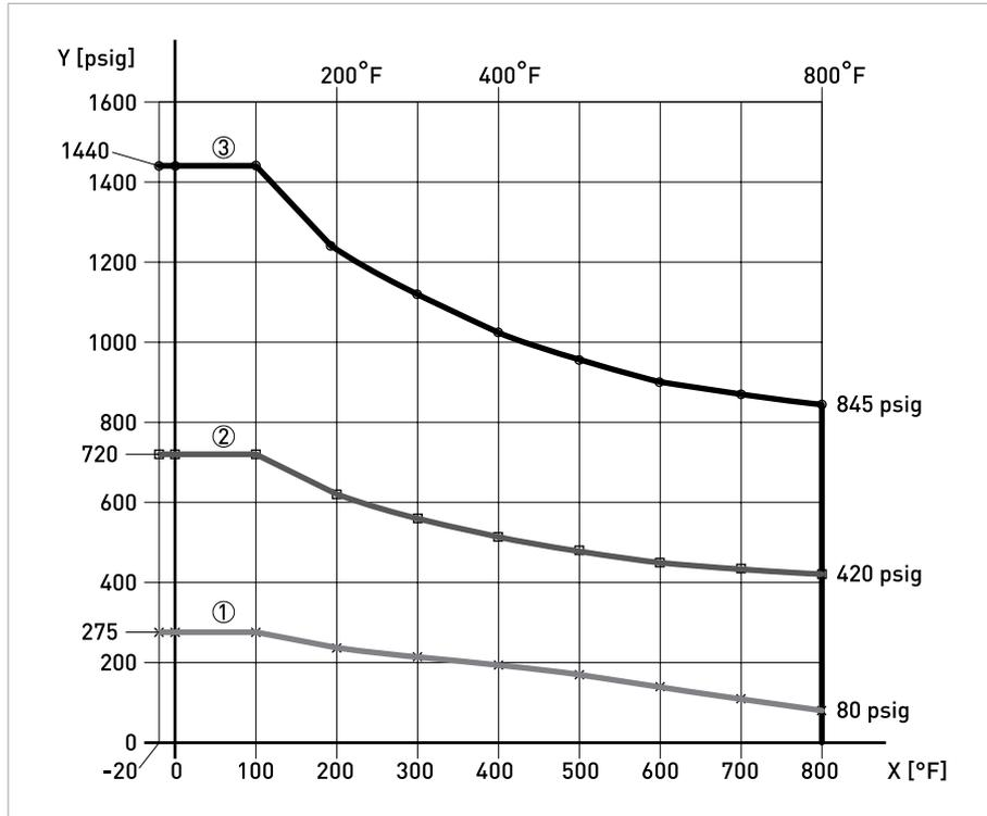
Figure 2-1: ANSI flange rating acc. to ASME B16.5 for group 2.2 materials
