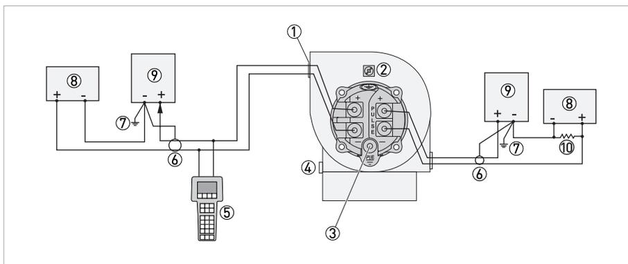
Figure 4-6: Wiring a flowmeter with a pulse output transistor switch (sinking) counter input with external power supply and pull-up resistor
