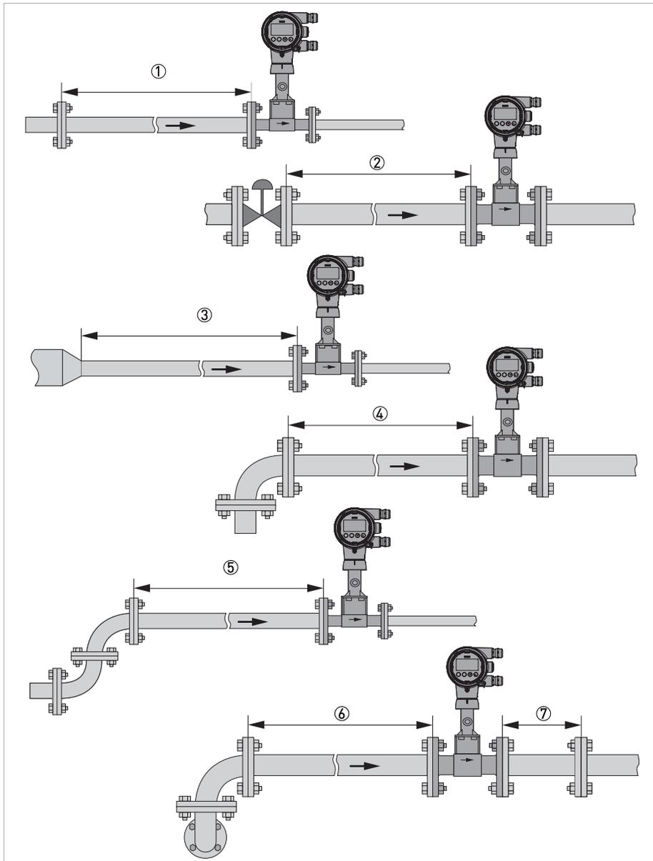
Figure 3-6: Minimum inlet sections
