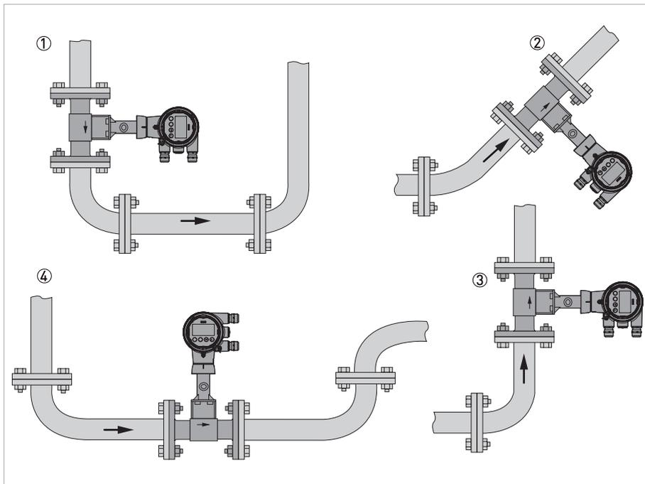
Figure 3-1: Recommended installation
